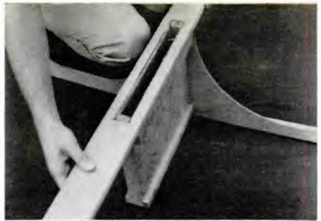
KEEL IS PRECUT to fit over the daggerboard trunk. Both ends are left oversize for custom fitting
